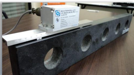
Granite straightedge calibration
