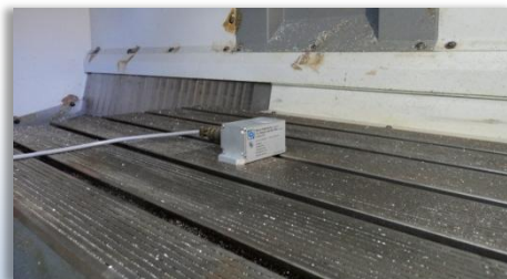
CNC machine levelling / calibration
